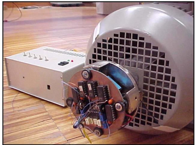
Fig. 5. Infra-red transmission system [12].
