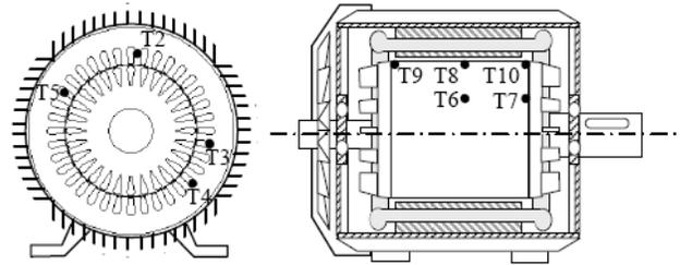
Fig. 4. Stator and rotor thermocouples location.
