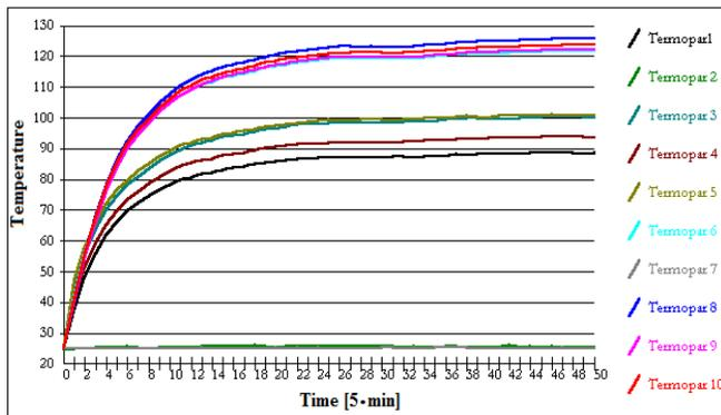
Fig. 6. The heating curves for a derating test corresponding to a PVU=4% and  $V_1=380$  V
