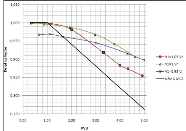
Fig. 7. Comparison of experimental Derating Factors (for three different values of positive sequence voltage) with NEMA MG1 derating curve.
