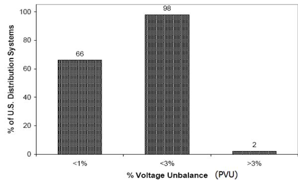
Fig. 1. Approximate "percent voltage unbalance" (PVU) in the U.S.A. Distribution System [5].
