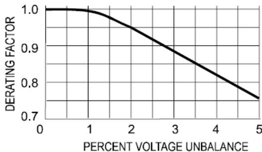
Fig. 2. Derating factor for squirrel cage induction motors due to unbalanced voltage. Standard ANSI/NEMA MG1 [6].
